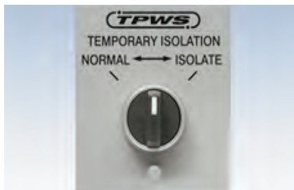
TPWS temporary isolation switch
